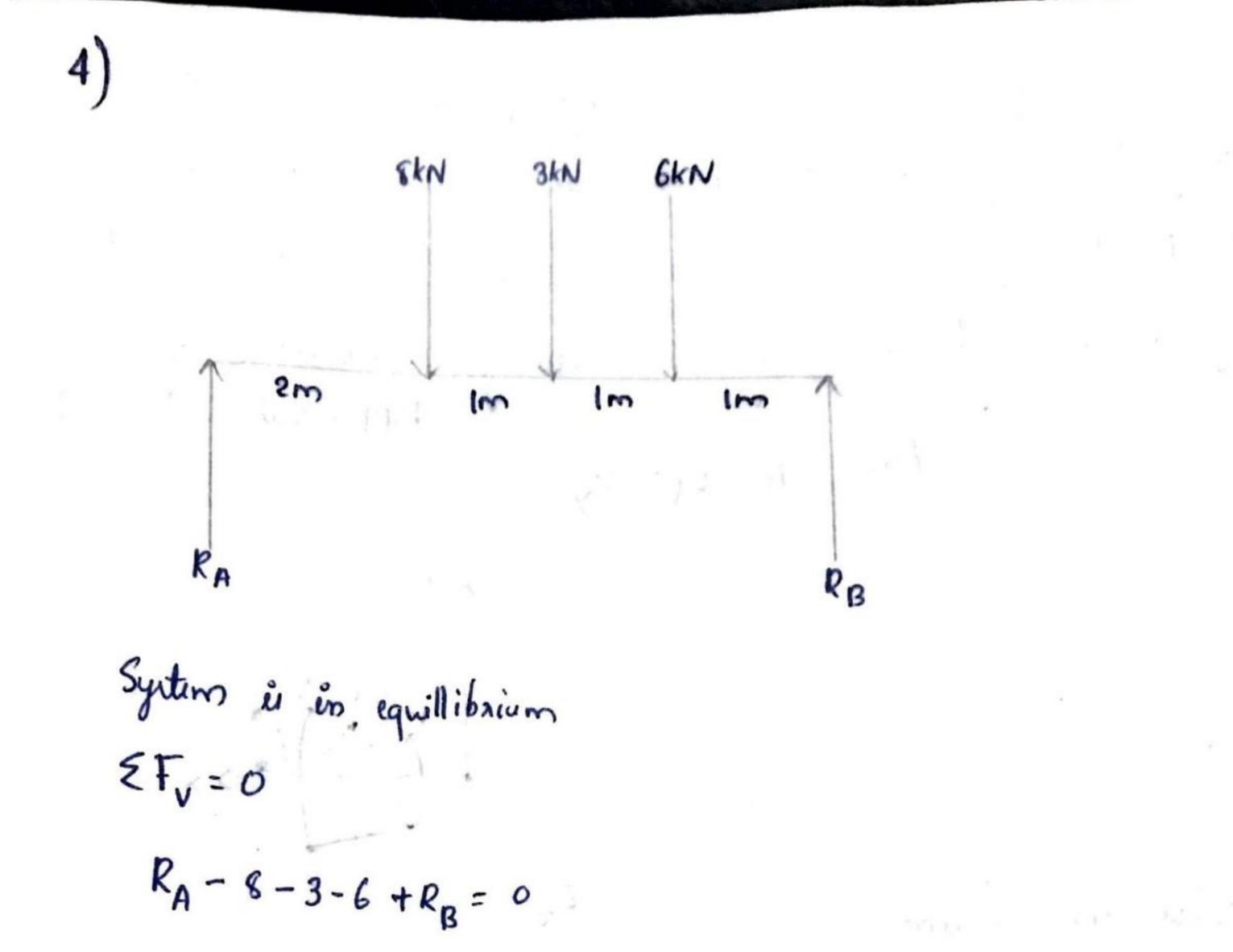
$R_{H} + R_{B} = 15 - 0$   $\text{Taking moment about A} \\ \leq M_{A} = 0$   $\sum M_{A} = 0 \quad 8 \times 2 + 3 \times 3 + 6 \times 4 \times 5 \times R_{B} = 0$   $16 + 9 + 24 \cdot 5 R_{B} = 0$   $5 R_{B} = 49$   $R_{B} = \frac{49}{5} = 9 \cdot 6 \times N$ Sub  $R_{B} \text{ in } 0$   $R_{A} + 9 \cdot 8 = 15$   $R_{A} = 15 - 9 \times N$
